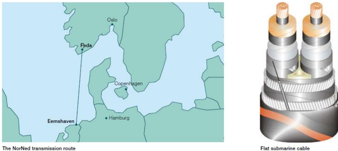
Figure 2. 3: The NorNed HVDC Transmission Link
